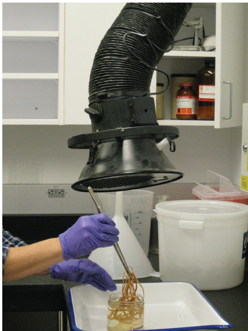
FIGURE 9.11 Fume extractor or snorkel.
